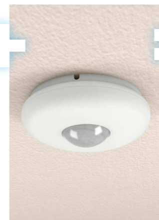
10b Motion detector together with door detector detects guest presence and activates Occupancy/Vacant function. This turns off unnecessarily lit lights.
