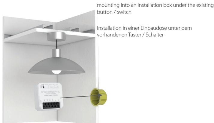
mounting into an installation box under the existing button / switch
