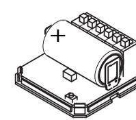
Insert a new battery, paying attention to the polarity of the battery.
