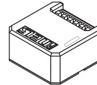
Replace the cover, pushing the tabs in the corners.
