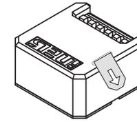
Batteries is inserted in the product. Before using for the first time, remove the insulating tape from the battery contacts by pulling in the direction of the arrow.
