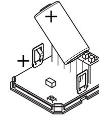
Remove the old battery and dispose of it in an environmentally friendly manner.
